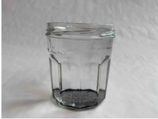
Figure 19. A typical sample of water drained from the kiln. Overnight a fine layer of microscopic biochar particles settles out, and the water remaining is extremely clear.
