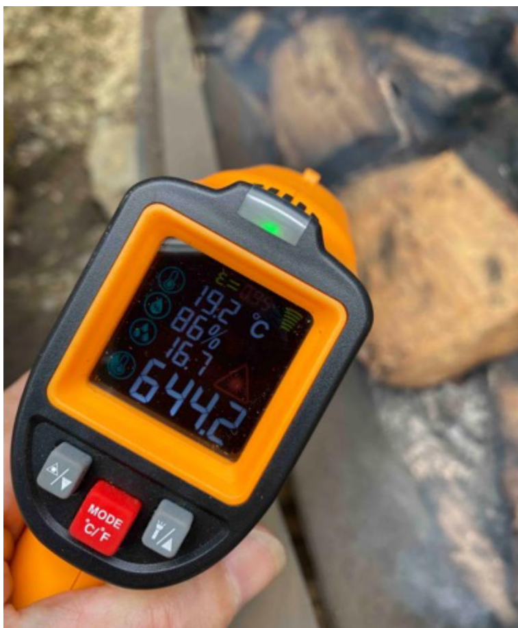
Figure 5. Temperature indicated using an EVENTEK ET323D infrared thermometer (range -50°C to +850°C)
