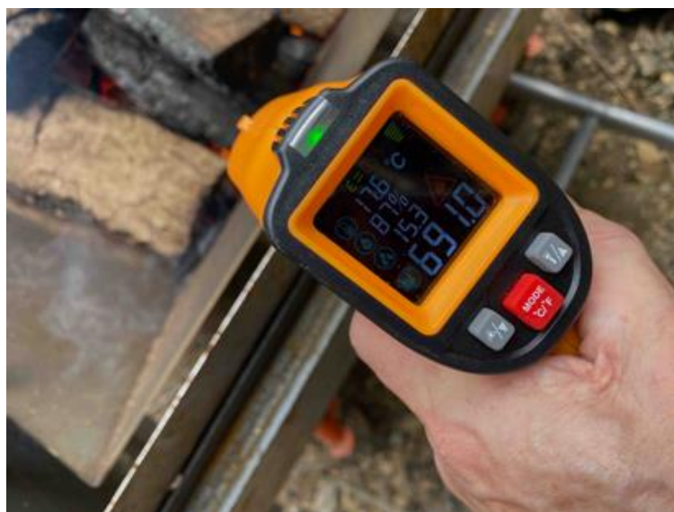
Figure 13. At this stage, the temperatures within the kiln can be routinely above 600°C. In this particular measurement: 691°C which is at the high end of target. With experience, temperatures within the kiln can be gauged by the colour.
