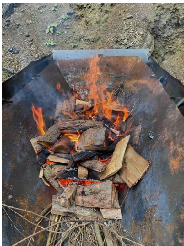
Figure 10. A layer of biomass added upon the original kindling material.
