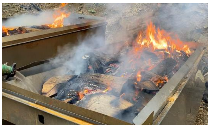
Figure 16. Pouring in quench water (gravity fed).
